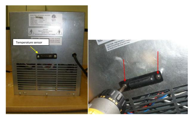
Unplug old temperature sensor (labeled: CN1) and plug new sensor in.
