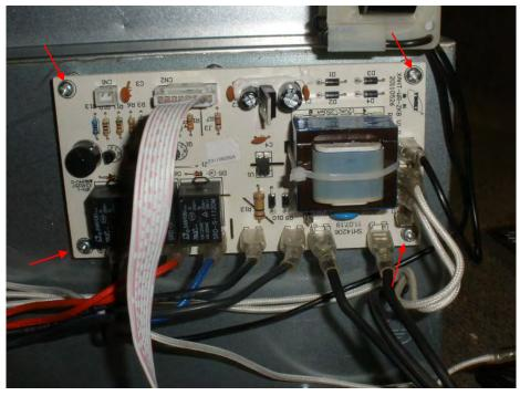
Put the new board in place. Disconnect 1 wire at a time from the old board and connect it to the appropriate location on the new board.
