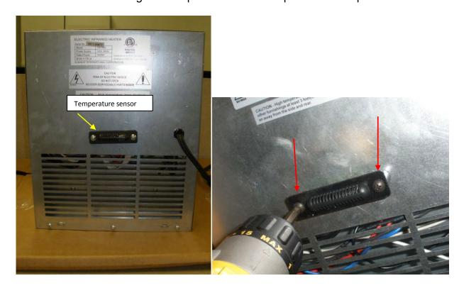
Unplug old temperature sensor (labeled: CN1) and plug new sensor in.
