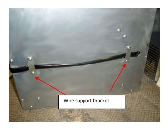
Remove back Panel by removing 9 screws. There are 3 screws on both side panels and on the bottom of the back panel.
