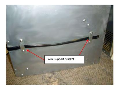
Remove back Panel by removing 9 screws. There are 3 screws on each side panel and on the bottom of the back panel.
