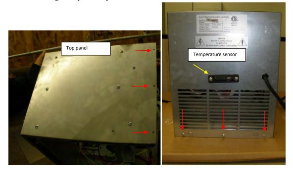
After Side and Back panels are removed, remove all the screws on the top panel. The mainframe can be pulled out to gain full access to fan.
