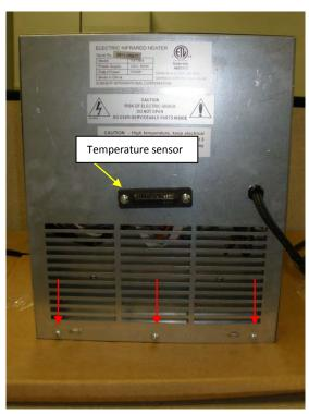
Remove 2 Screws holding the Temperature Sensor in place on back panel.
