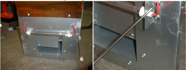
On the Right side of the heater you have a white ceramic wiring block, unscrew the wire that corresponds to the heating element you are replacing.
