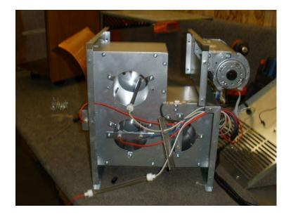
Disconnect 2 wires from the circuit board that come from the fan. They are labeled as: AC-N4 & FAN
